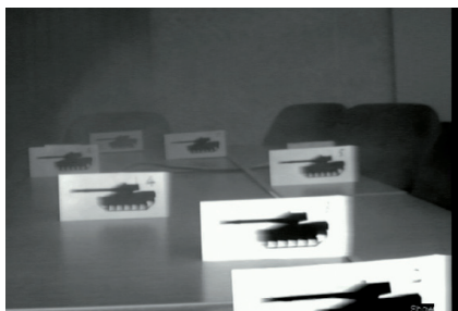
Image from a VIT55 Fog Camera looking into the same smoke-filled room.
